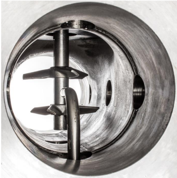
Figure 1. Photograph of an inline mixer with a polymer injector directly upstream of dual hydrofoil impellers.
