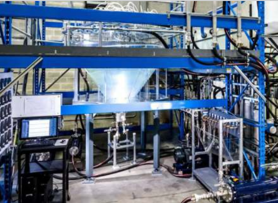
Multiphase Separation Flow-Loop
